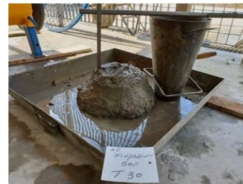
Slump Test T30
