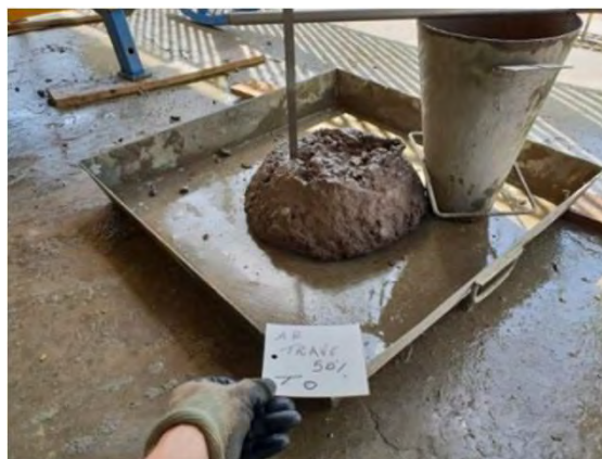
Slump Test T0
